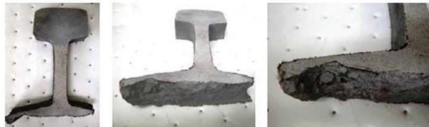
Figure 6: Different views of a section of 100 lb rail showing severe corrosion at the base of the rail (Francisco & Gabriel, 2007). Reproduced with permission from the National Academies Press.
